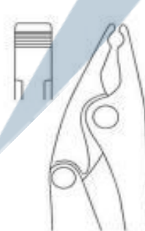
11-01-0420 Plate Bending Pliers 14.5 cm / 5 ½"
